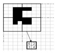
Figure 4: 32x32 to 8x8 image conversion using 4x4 block size.
